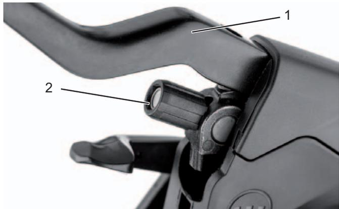
**Illustration 28:** Brake lever (1) of the hydraulically operated rim brake with setting bolt (2)
