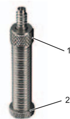
**Illustration 26:** Dunlop valve with union nut (1) and rim nut (2)
