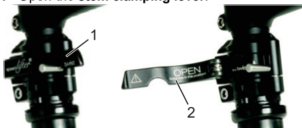
Figure 39: Open (2) and closed (1) stem clamping lever – by.schulz speedlifter used as an example
