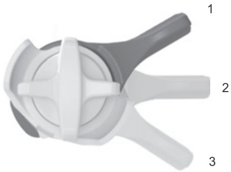
Figure 59: FOX compression adjuster on the rear frame damper with OPEN (1), MEDIUM (2) and HARD (3) positions
