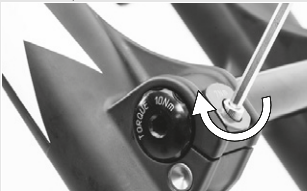
Figure 18: Tightening the securing clip
