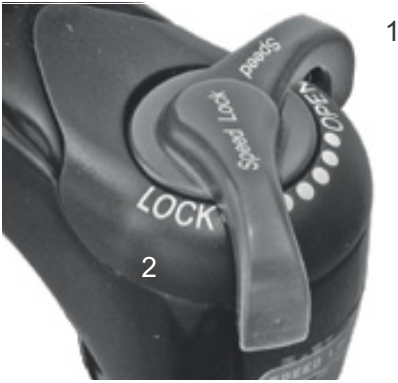
Figure 55: Suntour compression adjuster with OPEN (1) and LOCK (2) positions
